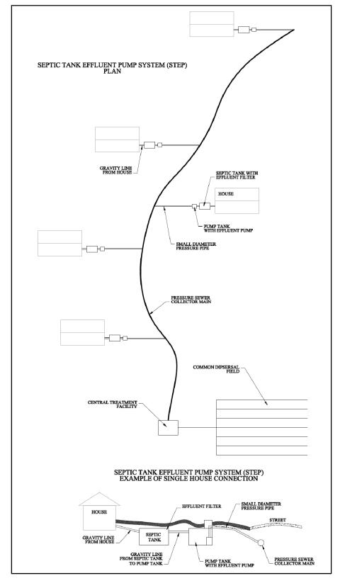
Figure 3-3 Diagram: Other Collector Systems, Showing Individual Connections
