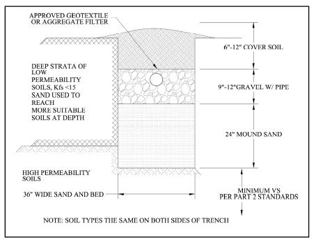
Figure 3-33 Above Ground Sand-lined Trench
