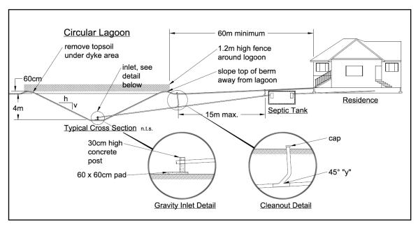
Figure 3-40 Circular Lagoon (Top View)
