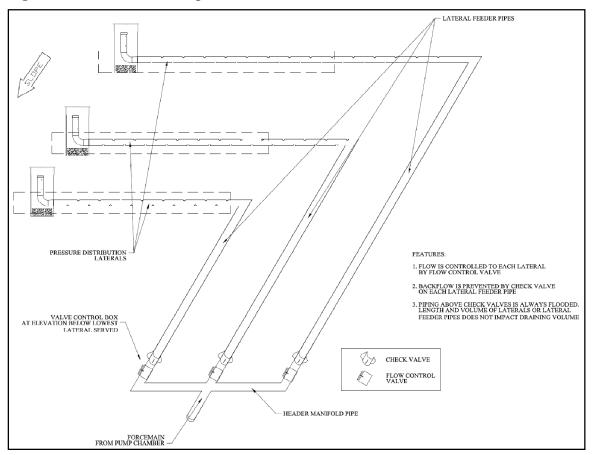
Figure 3-19 Short Downslope Header Manifold, with Check Valves.
