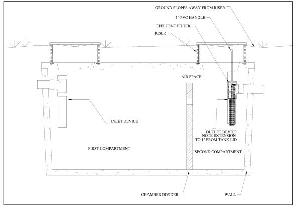
Figure 3-5 Flow in a Septic Tank.
