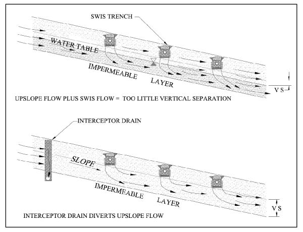
Interception drains act to divert water flowing on the surface and below the surface from upslope to the discharge area, improving vertical separation and in-soil treatment.
