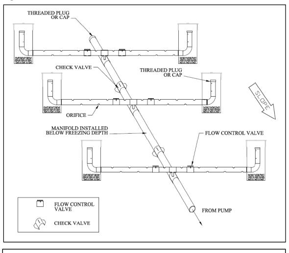
Figure 3-16 Tee to Tee Manifold, with Check Valves.
