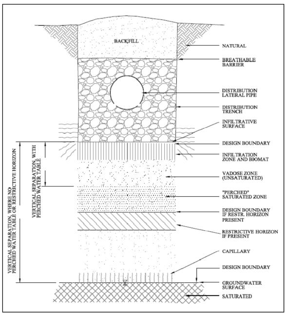
Figure 3-7 A SWIS Trench System, Showing Terminology
