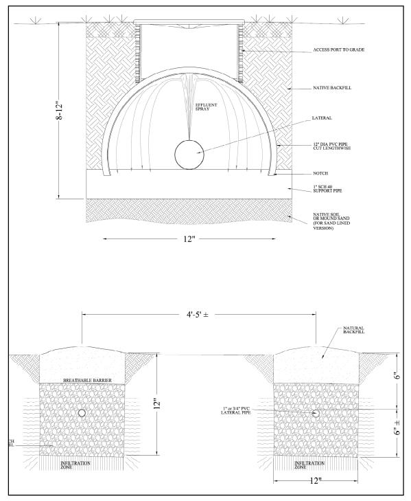
Figure 3-25 Shallow Narrow Drainfield Cross Sections
