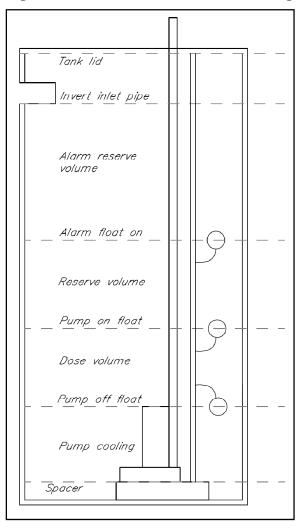
Figure 3-21 Schematic of Demand Dosing Terms
