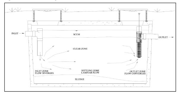
The septic tank provides settlement/flotation, together with some anaerobic treatment and digestion of sludge *(see Figure 3-5)*. Settlement is improved in tanks that have a shallow and long flow path, and settlement is a function of surface area in relation to flow.
