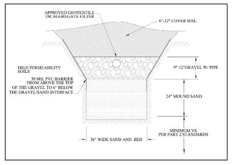
Figure 3-32 Sand-lined Trench to Reach Suitable Soil at Depth
