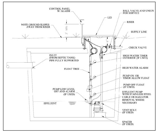
In cases where a supply line exiting as shown in Figure 3-20 will freeze, loop supply line back down from riser and exit at greater depth.
