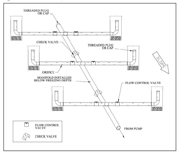
Figure 3-17 Cross Manifold, with Check Valves.
