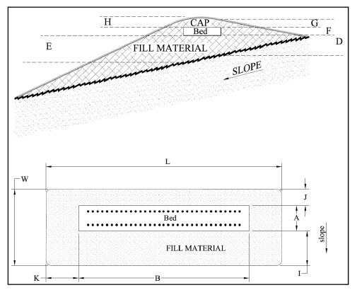
These systems should be constructed perpendicular to the slope, following contour, and should be long and narrow addressing LLR standards. LLR should be considered for the area directly under the systems and the receiving area (7.5 m (25') downslope on a sloping site, 7.5 m (25') to all sides on a site with slope under 1%).
