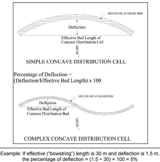
Figure 3-36 Calculation of Effective Bed Length on Site with Concave Contour
