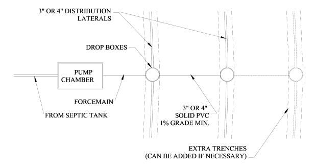
Figure 3-13 Sequential (Drop Box) System (Top View)
