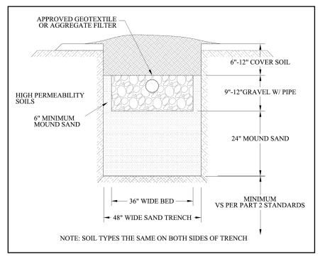
Figure 3-31 Sand-lined Trench with High Permeability Soils to Surface, Option 2
